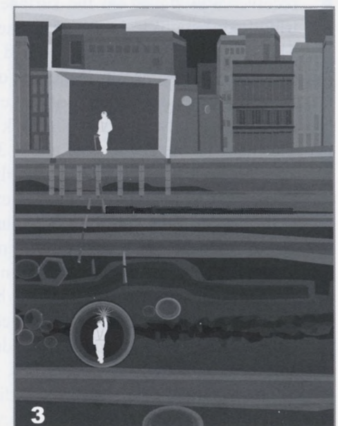
1 A technician takes reading on the surface as another places the sonde in the sewer. 2 If sewer wasn't located, it could be damaged by builders. 3 As reading is taken, there is interference from other sources such as hydro, gas and rebar in the building's floor.
